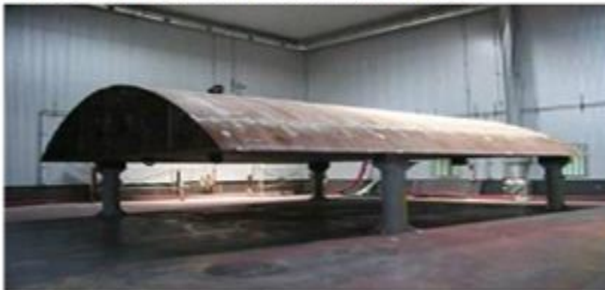
Pre-coating treatment of construction block
