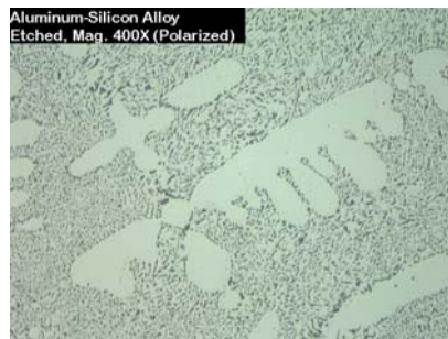
Figure 4. Aluminum-silicon alloy solidification microstructure
