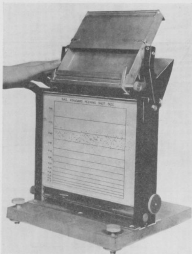
FIGURE 1. Mattson apparatus for determining size and distribution of peening shot.
